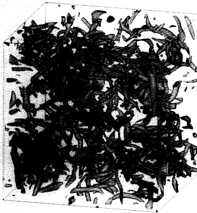
Fig. 1. – Isosurfaces of (a) the vorticity magnitude and (b) the Laplacian of pressure in isotropic turbulence. The thresholds are set so that each of them covers 5% of the total volume.
